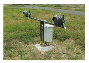
The monitoring of targets is also extended to vehicles that move on the peripheral roads enter directly that the runways. In this case the double microwaves sensors are located near the marker of holding position of the roads. The system controls traffic vehicle with proper traffic lights to prevent possible errors of the drivers.
